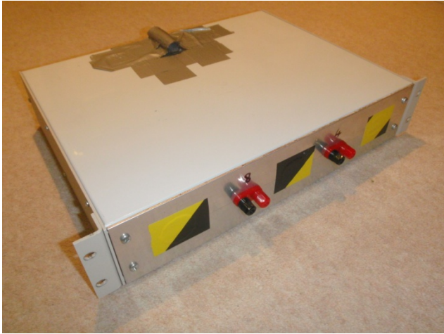
Figure 2 Front of Sound Source - Three apertures covered with vinyl tape to prevent fans pressure back loading the transducers
