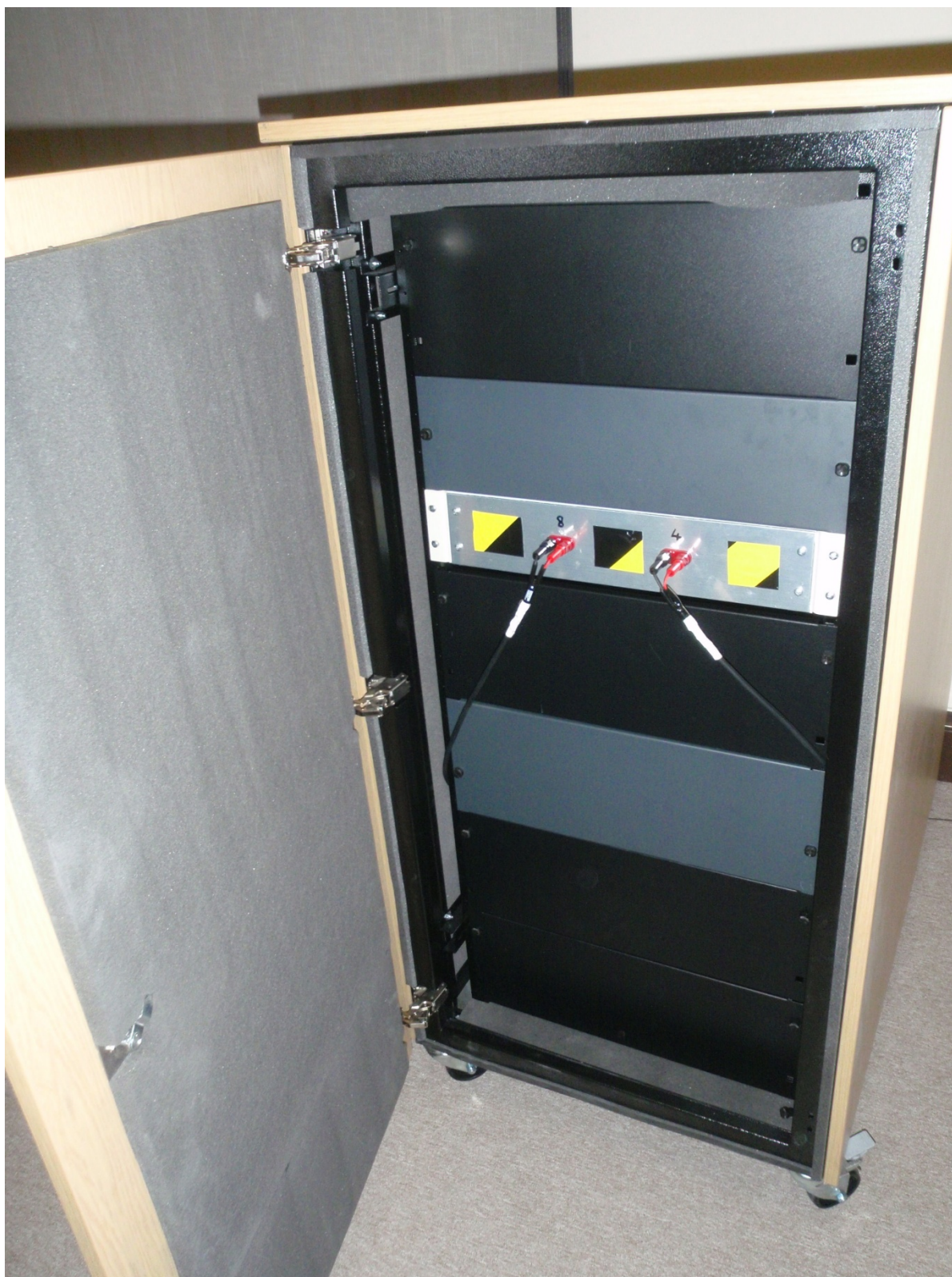
Figure 5 Sound source fitted to a cabinet with blanking plates fitted
