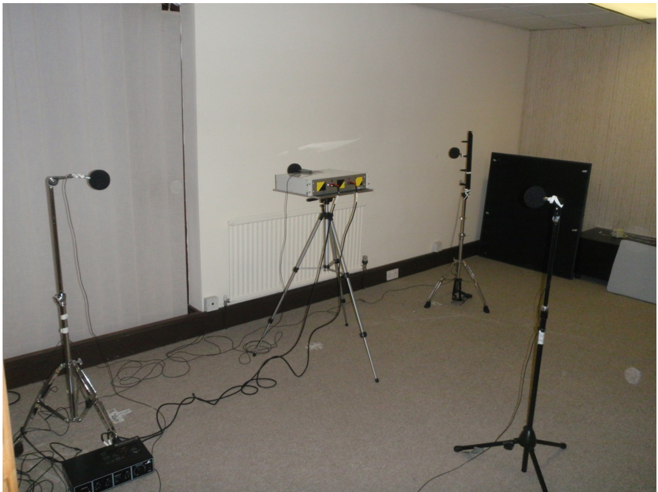
Figure 4 Microphone Layout for setting the sound source levels
